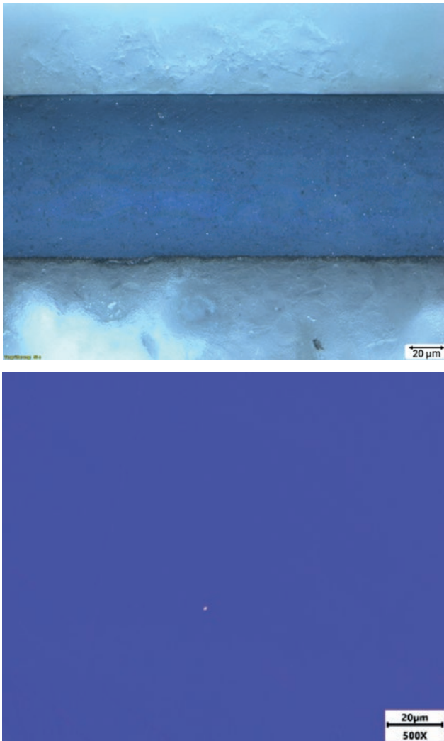
Fig. 4: Inclusion analysis of 4 mm x 0.1 mm tube in longitudinal direction using 500x magnification. Upper: Analysis by Admedes. Lower: Analysis by MeKo.
