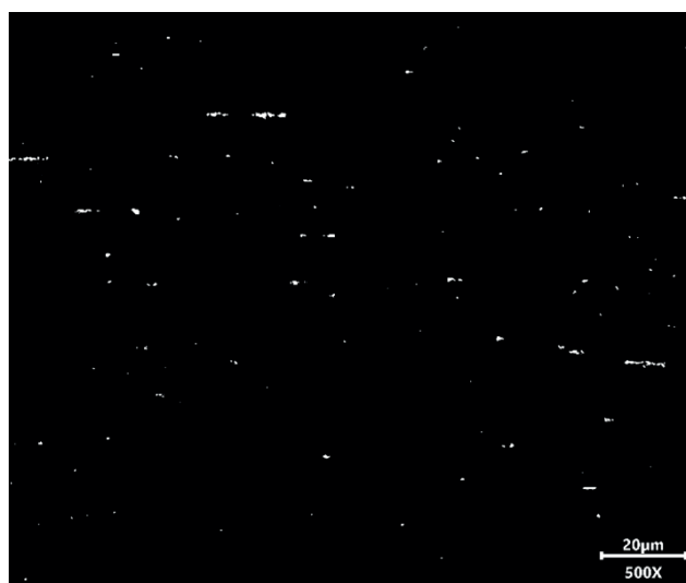
Fig. 3: Inclusion analysis of 2 mm x 0.22 mm tube by Euroflex in longitudinal direction using 500x magnification. Upper: Analysis by Admedes. Lower: Analysis by MeKo.
